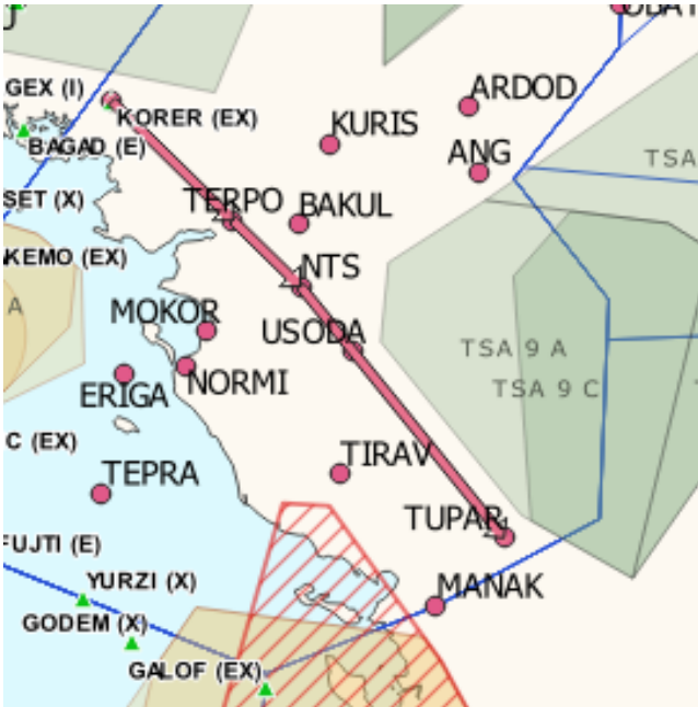
Transition to GAT at KORER, mandatory GAT trajectory from KORER to TUPAR, free GAT trajectory afterwards.
