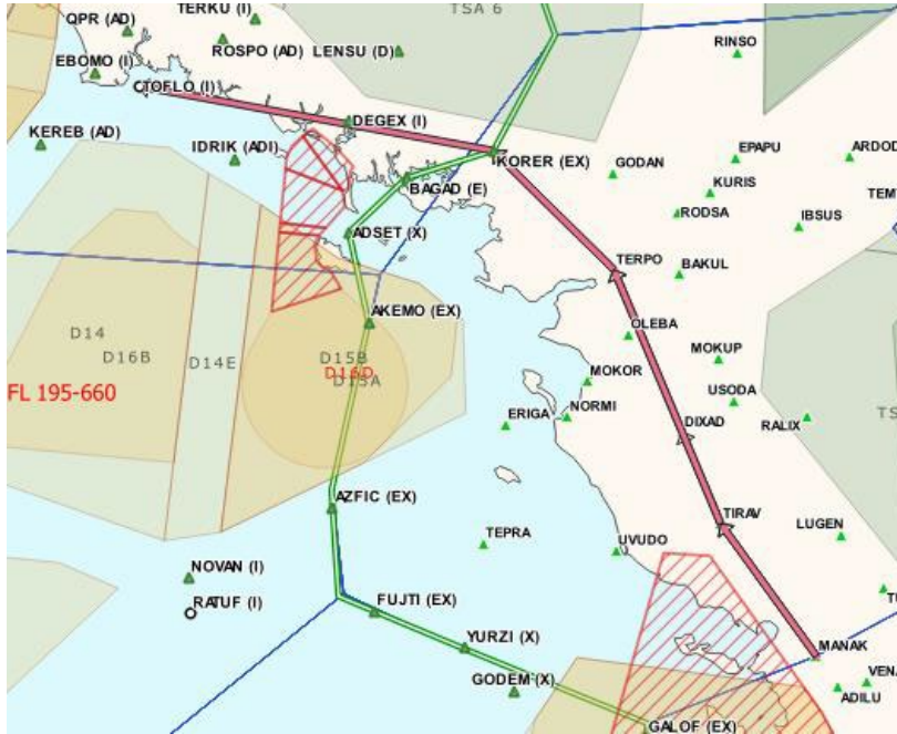
Transfer to OAT at the TOFLO point, free GAT trajectory before MANAK, GAT trajectory mandatory from MANAK to TOFLO, free OAT trajectory after TOFLO.
